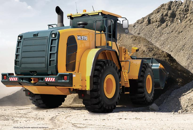
308 HP (230 kW)/2,100 rpm | 24,000 kg/52,909 lb | 4.2 m<sup>3</sup>/5.5 yd<sup>3</sup>
