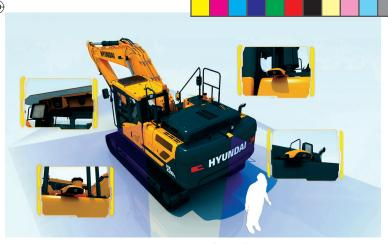
The AAVM option combines images from four external cameras to provide 360° virtual operating view.
