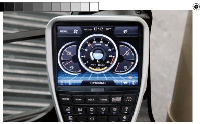
The 20.3 cm (8 in), touchscreen automotive-quality monitor with haptic remote control provides easy access to almost all systems and functions.
