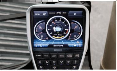
The 20.3 cm (8 in), touchscreen automotive-quality monitor with haptic remote control provides easy access to almost all systems and functions.
