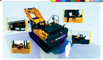
The AAVM option combines images from four external cameras to provide 360° virtual operating view.
