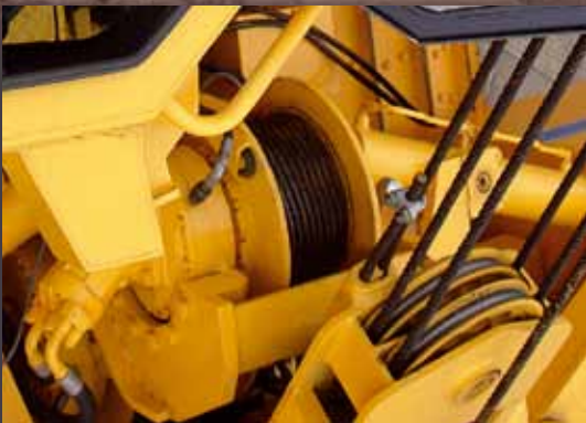
Side boom and hook are controlled by hydraulically driven heavy duty winches.
