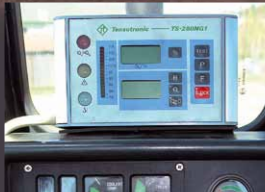
Optional electronic safe load indicator (ESLI) displays necessary load handling information.
