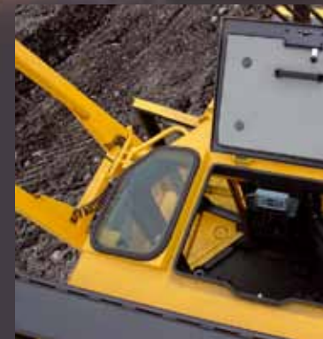
Cab roof window provides full view for emergency operations while the emergency operator's safety.
