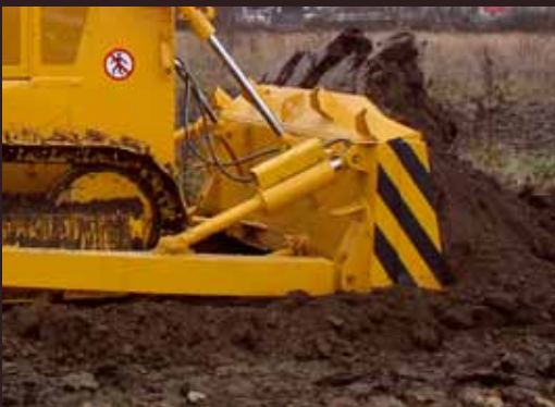
Semi-U blade of 4.28 m 3 (5.6 yd 3 ) (STD)
