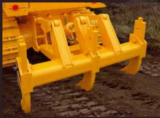
The optional three-shank, parallelogram type ripper is ideal for ripping in tough material.
