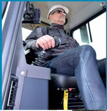
The all new hexagonal cab provides 30% more space and features full sound suppression. The cab is FOPS certified while the machine incorporates an <u>additional two post</u> ROPS protection system. Cab features include:
